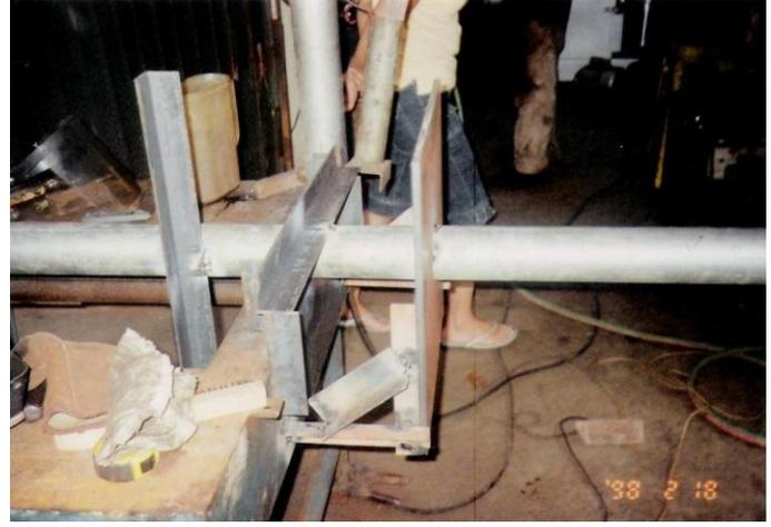
Figure 3: Internal buoy structure with 9 foot, 3 inch diameter pipe and two angle bars for support. The yellow panel is the keel (left).
